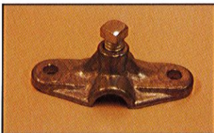
Blade Saddles - Half Circle Product Size and Code # 1/2" # 1760 12mm # 1762 3/8" # 1764 10mm # 1766
