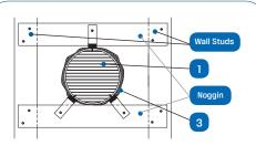
FACE FIXING: Alternative fixing method Kilargo Intumescent fire damper supported by noggins fixed to studs
