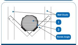
FACE FIXING: Alternative fixing method Kilargo Intumescent fire damper supported by external Rondo angle hung between studs.
