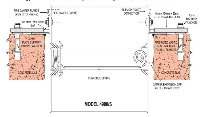
NOTE: For any damper 300mm x 300mm or less only two clamps are required on opposite sides of the damper. If the damper or bank of dampers are larger than 300mm x 300mm then there must be at least four clamps - one on the centre of each side. If any side of the damper exceeds 600mm then an additional clamps are required at nore more than 300mm centres.
