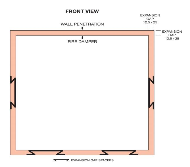
Expansion gap spacers come fitted to Bullock Fire Dampers to ensure the damper is centred within the penetration, they will not sag like other insulated products leading to gaps above the damper over time.
