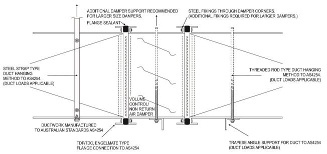
NOTE: Should damper blades drag upon the damper frame (Models 6700/6500) this indicates frame misalignment and the installation is incorrect. Algin frame correctly before continuing damper test. Damage to the dampers vital blade sealing system may render the damper inoperable. The damper would then need to be returned to the manufacturer for repairs at a cost to the installer. Should operational checks show correct installation, proceed to connect actuator to drive shaft.
