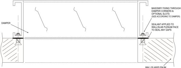
NOTE: Should damper blades drag upon the damper frame (Models 6700/6500) this indicates frame misalignment and the installation is incorrect. Algin frame correctly before continuing damper test. Damage to the dampers vital blade sealing system may render the damper inoperable. The damper would then need to be returned to the manufacturer for repairs at a cost to the installer. Should operational checks show correct installation, proceed to connect actuator to drive shaft.
