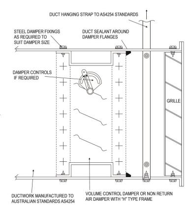
**NOTE:** Should damper blades drag upon the damper frame (Models 6700/6500) this indicates frame misalignment and the installation is incorrect. Algin frame correctly before continuing damper test. Damage to the dampers vital blade sealing system may render the damper inoperable. The damper would then need to be returned to the manufacturer for repairs at a cost to the installer. Should operational checks show correct installation, proceed to connect actuator to damper drive shaft.
