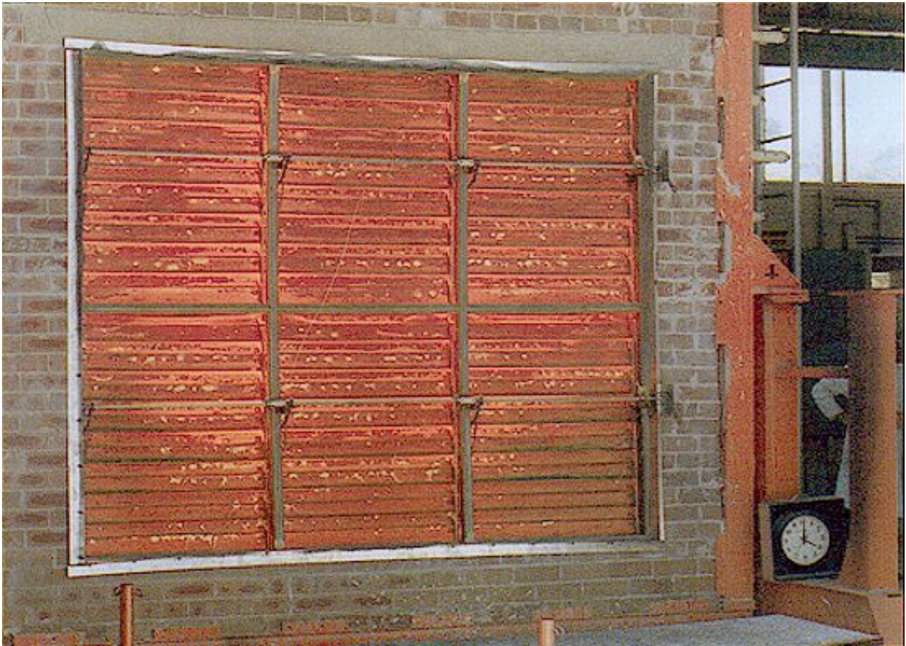
Prefco / Bullock combination Air / Smoke / Fire Damper Fire Tested for a 4 hour rating to AS1530.4 - 1975, BS476: Part 20 - 1987 Fire Tested for a 3 hour rating to UL555. Performance leakage test to UL555
